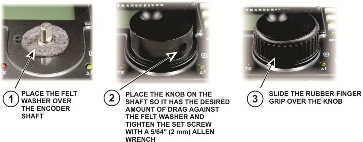
Figure 20. Mounting the VFO Knob.
