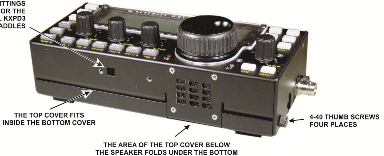
Figure 49. Test Fitting the Top and Bottom Covers Together.
